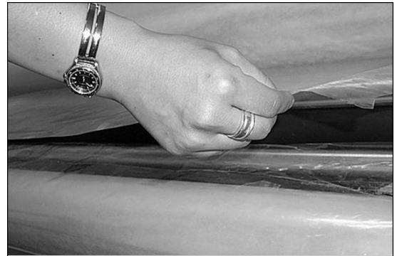
Tacking laminate from top roll to exposed adhesive on bottom roll
