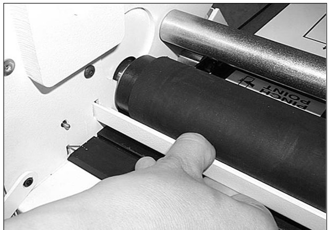
Push bar towards left side of the machine
