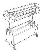
2. Look for the marks on the printer for correct installation.
