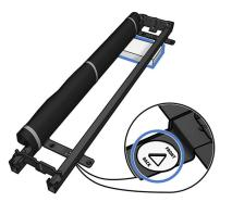
4. Place leg into slot on cross brace with long side of foot as shown.
