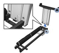
5. Attach leg to cross brace with 3 screws at the inside of leg.
