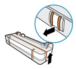
7. Remove the 2 spindle tapes and retainers.
